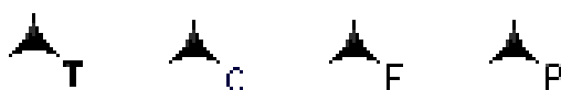
Figure 3.1: Depending on the type of object beneath the cursor, a letter is shown next to the arrow. From left to right: Track, Clip, Fade, Plugin.
