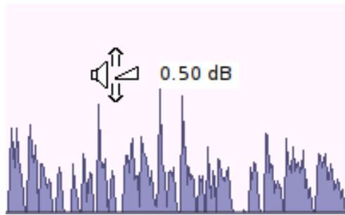
Figure 5.1: The cursor changes to a gain symbol during the [G] action.
